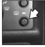
The rear window defogger uses a warming grid to remove fog from the rear window.
